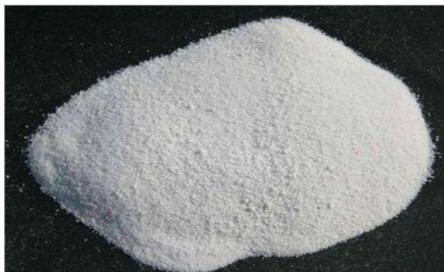
Figure 18: Expanded perlite powder [130]
