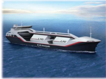
Figure 10: Conceptual design for two LH 2 carriers from Kawasaki Heavy Industries: a) large and b) small [43]
